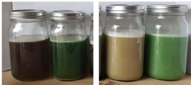
Temetry® LFR® 9.5 fl oz/A in Begin® (left jar) and 10-34-0 (right jar) 24 hours after mixing.
