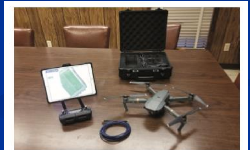
Figure 1: Complete real-time mapping system: DJI Mavic Pro, case, Apple iPad, DroneDeploy and an extra-long lightning to USB cable.
